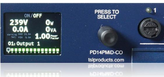
The output will now switch **OFF**. The output indicator will turn off to show this as will the front and rear output LEDs
