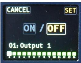
Rotate the encoder until **OFF** is highlighted then push the encoder to select.
