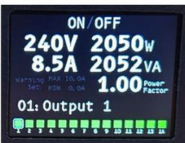
By rotating the encoder to the right, the output switches and settings can be accessed for each individual output, 1 to 14.
