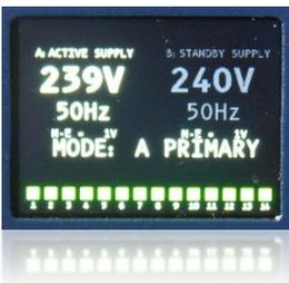
This monitoring mode displays the voltage and AC frequency of each mains input with the active supply being highlighted and indicated.
