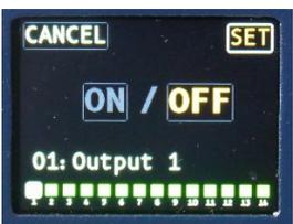
Rotate until **SET** is highlighted then push the encoder to select.
