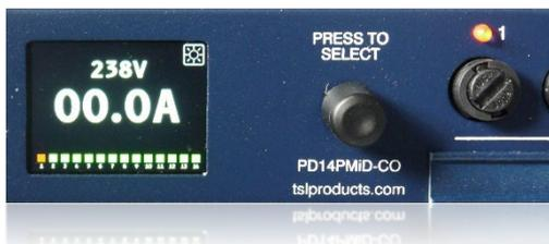
In the event of a fault on any output which causes a front panel fuse to blow the LED associated with that output will be **RED** if the outlet is switched ON.
