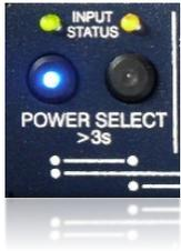
To set the Primary input - which is the preferred active input – hold and press the **OFF** button together with the desired input (either A or B) until the **BLUE** button LED illuminates.
