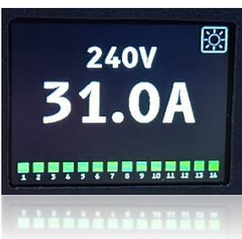
On this page, the voltage of the active input and the sum of the current load for all outputs are displayed. Display brightness can also be adjusted in this mode, as indicated by the icon on the top right corner.
