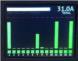
In this mode, the current load of each output channel can be monitored with the overall load displayed in the top right corner of the display.
