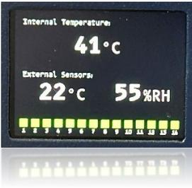
This page shows the internal temperature of the unit, and if connected, the ambient external temperature and relative humidity percentage measured by an external sensor.
