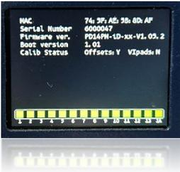
Select the unit information screen front panel menu and check the Firmware version matches the expected upgrade version.
