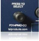
The unit can be operated from the front panel using the rotary encoder next to the display. Each monitoring mode can be selected by rotating the encoder to either side and selections can be made in menus by pressing it.
