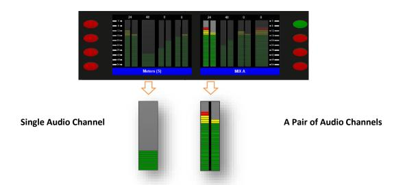
This allows the SAM-Q-SDI to display Mono and Stereo audio sources simultaneously.
