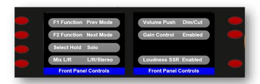
To modify any of the default functions, simply select the control you wish to modify and use the large rotary encoder to select your preferred function.
