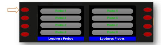
Select button 1 to select the Probe Type and rotate the Large Encoder to select the program configuration you would like the Probe to measure.
