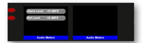
To adjust either setting, simply push the corresponding Source Select button and use the large rotary encoder to enter the required value. To apply the new setting simply push the large encoder or the corresponding Source Select button once more.
