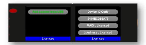
To load a license, simply copy the file supplied by TSL into the root directory of a USB thumb drive, insert it into the front panel of the SAM-Q-SDI and select 'Add License from USB' using Source Select button 1.
