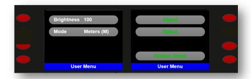
To change a setting, simply press the corresponding Source Select button, enter the new value by rotating the large encoder and then apply the change either by pressing the source select button or by pushing the large encoder to finish.
