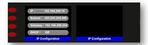
Use Source select buttons 1 through to 3 select and enter the required IP address, Subnet and Gateway respectively.
