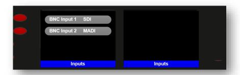
To switch either BNC Input between SDI and MADI, select the Audio Select button for the corresponding BNC Input and rotate the large encoder.
