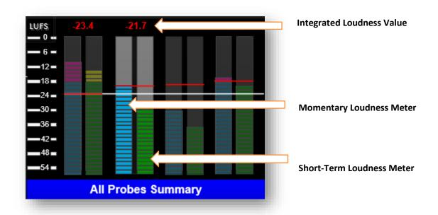
Selecting a different loudness probe for monitoring causes the previously selected loudness mode to be deselected automatically.
