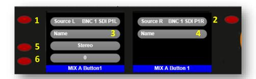
Selecting Stereo mode (Item 5) will cause a dual audio level meter to be displayed for the respective source in the chosen Mix Group. Both Left and Right sources (Items 1 and 2 above) will be audible when selected by the User (see below).
