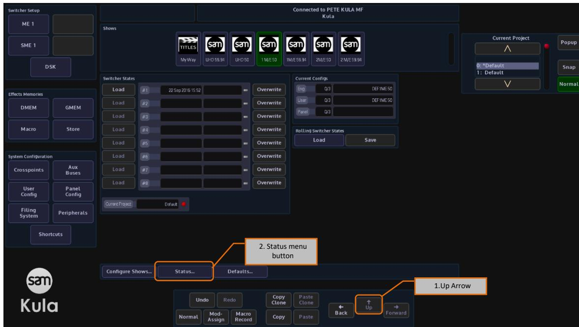
Press the 'Status' button near the bottom of the screen and the page below will appear.
