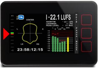
phase" is a signal where the mono sum would be less than the higher of the left and right signals. Signals which are predominantly "in phase" have a green marker in the upper half of the range. Fully correlated signals such as double mono read on the +1 mark. Signals which are "out of phase" are shown with a red marker in the lower half of the range.
