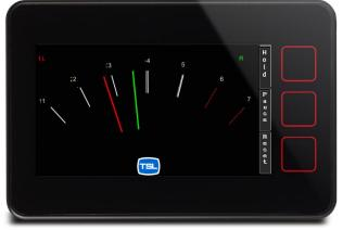
The Dual mode allows a single moving coil arc to display two signals by using a dual Needle Concept. The specific signals displayed depend on the signals routed in the Matrix Output Assign folder e.g. Left/Right or M/S.
