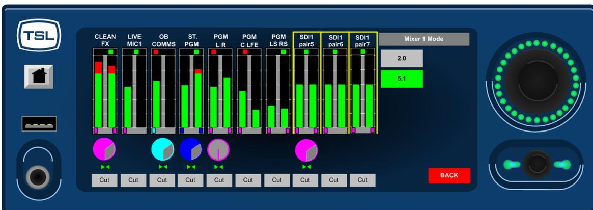
As previously described, Mixer 1 can operate in either Stereo or 5.1 modes. The mixer can be switched via the illustrated menu above.
