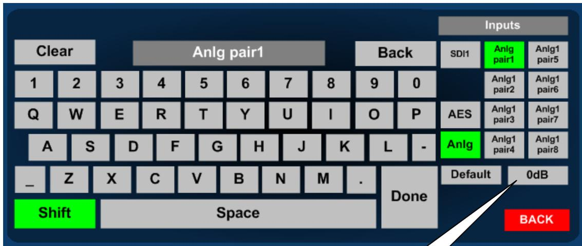
Press to access Input Trim for low level or unbalanced analogue audio
