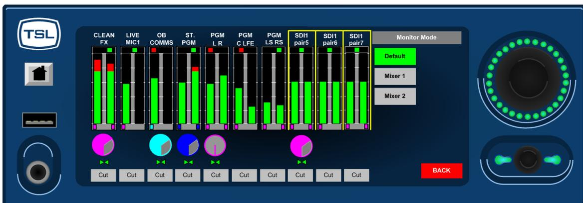
In **Default** mode the operator would normally hear the output of whichever mixer is currently shown on the touchscreen. The user can choose to hear either **Mixer 1** or **Mixer 2** permanently regardless of the mixer under direct control.
